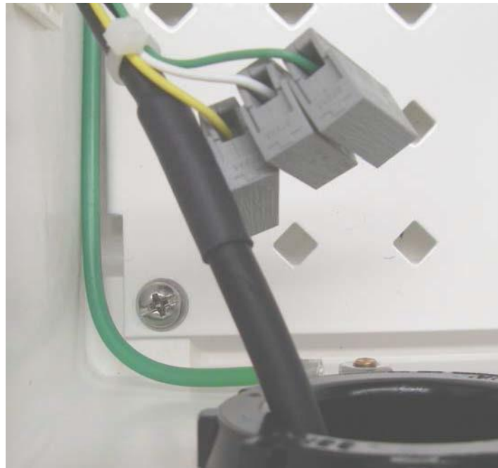
Figure 4-1 CC5MPX Connector Layout
