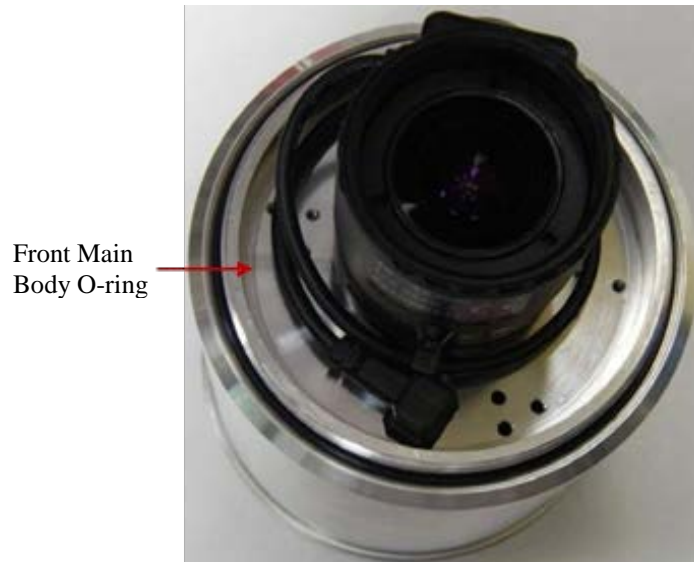
Figure 19-3 Front Main Body O-ring
